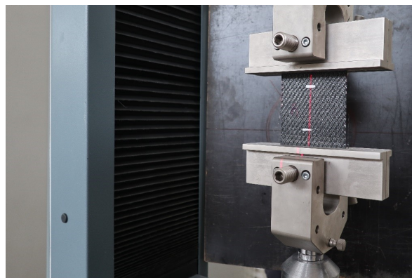
Figure 1—Test arrangement of product similar to geotextiles
