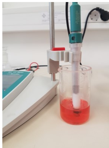
Figure 2—Measuring pH value in Hank's solution
